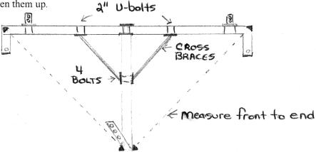
• Next you can bolt on the 2- wing mounting brackets with 2 - 1/2 x 3 1/2" bolts and lock nuts. After they are on you can bolt on the 10' long wings with 2 - 1/2 x 3 1/2" bolts and lock nuts. The end with just a hole drilled into it is the end that attaches to the main frame.
