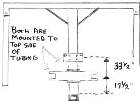
• You are now ready to mount the wick tubes with the 3" u-bolts and flange nuts. (remember for maximum wicking action they must be mounted with the fill cap to the top and ropes sticking straight ahead **not** pointing down toward the ground. The 3" u-bolt just slips around the 3" pipe and then it gets fastened onto the muffler clamp. **Do not** over tighten, they should be tight but not squeeze the pipe.
