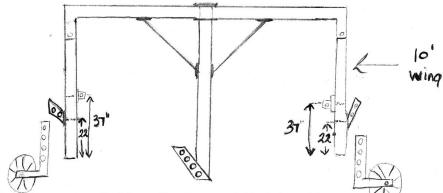
• Next you can put on all of the muffler clamps with 2" u-bolts and flange nuts. It is important to keep these measurements fairly accurate. (You will have trouble mounting your tubes later if you don't) On the main frame, measuring from the end (all measurements are to the center of the clamp, and they get bolted onto the underside of the tubing) they are 6", 58", 66", and 118".
