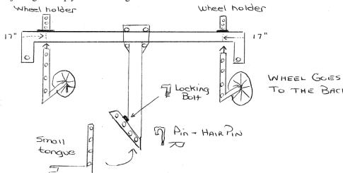
• Next you can put on the cross braces. They are joined together on the tongue with 4-3/8 x 3 1/2" bolts and flange nuts, and fastened to the main frame with 2 - 2" u-bolts and flange nuts. Before tightening them measure from the front to the outside ends. (this is done to make sure that when the unit is finished it will pull straight) If they do not measure close to the same you can adjust your cross braces to correct this and then tighten them up.
